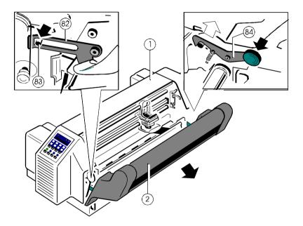
**Note:** On the ledge covering the blade in the **printer with cutter** is a label that cautions against touching the blade.
