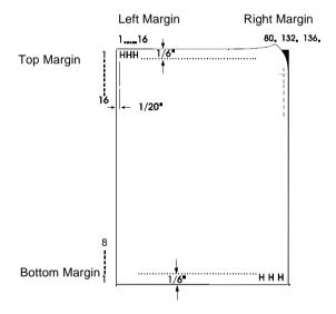
The bottom margin indicates the last print line. Going beyond this margin automatically initiates a form feed. The bottom margin is always set in steps of <sup>1</sup>/<sub>6</sub>".
