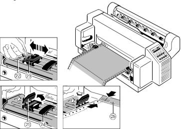
**Note:** The pins of the tractor must be centered in the transport punches of the paper.
