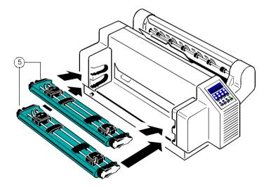
Insert the paper as shown in the illustration; the top edge of the paper must be equal with the top of the tractors or maximum up to two transport holes above the tractors. The left perforation should be aligned with the center mark on the plastic plate.
